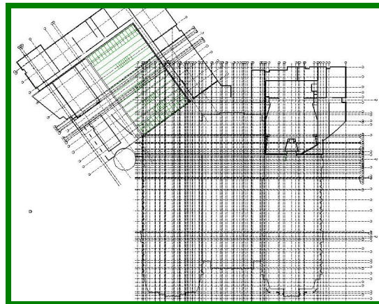
Figure 24 Autodesk Revit Building 9.1 - Structural Grid
